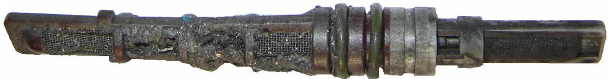
Example of contamination collected on inlet side of orifice tube requiring system flushing
