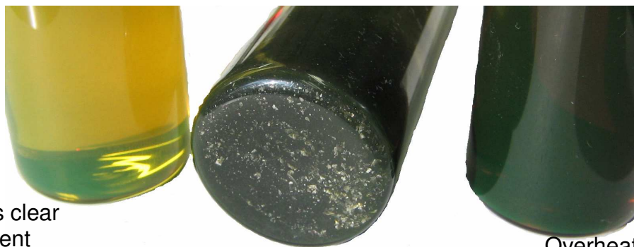
Contaminated oil with metal particles will require system flushing
