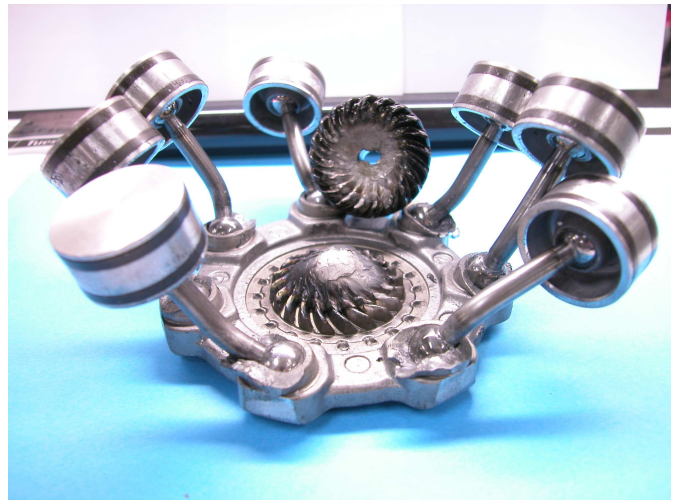
Overheated center ball and gear set
